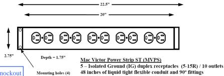
Now available with ½" EMT knockout on back for mounting over single gang flush mounted junction boxes.
