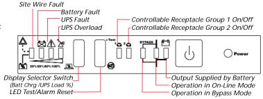
Indicator and control panel for the Sinergy S II Series UPS
