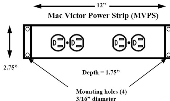
Now available with 1/2" EMT knockout on back for mounting over single gang flush mounted junction boxes.
